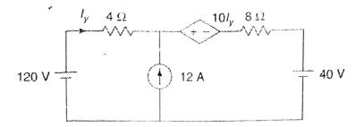
Q3 a Find the value of the resistance R<sub>1</sub> in the following circuit, for maximum power 10M transfer, and calculate the maximum power.
