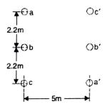
Q 3 a) A single circuit 460 kV line using two bundle conductors per phase as shown in Fig.
