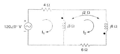
b For the given network draw oriented graph and write the (i)reduced incidence matrix 10M (ii) tieset matrix and (iii) fundamental cutset matrix.
