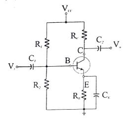
Q3) Perform small signal analysis over a BJT CE amplifier with voltage divider bias using the h-model. Derive an expression for current gain, input impedance, voltage gain and (10)output impedance.
