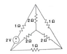
Q3 a Determine the Y parameters of the network shown . 10M  $\,$  0.5 F
