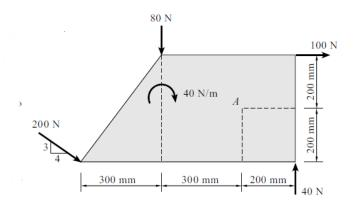
c) Determine the "x" and "y" coordinates of the Centroid for the shaded area shown.
