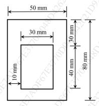
(b) Both machine components AC and PS are acted upon by a tensile load of 50 kN. Find the ratio of their strain energies. Take  $E = 2E5 \text{ N/mm}^2$ .
