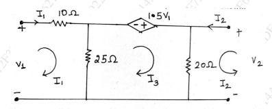
(b) Find Z parameters for the network shown. Check whether condition of Reciprocity is verified?
