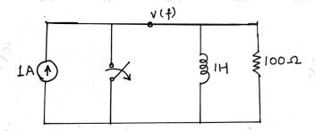
(b) In the network shown in figure the switch is closed and steady state is attained. At at t=0, switch is opened. Determine the current through the inductor.
