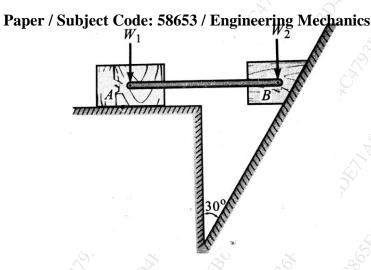
b. For the system shown in fig. if the collar is moving upwards with a velocity of 1.5m/s. Locate the ICR for the instant shown. Determine angular velocity of rod AB, Velocity of A and velocity at the midpoint of AB.
