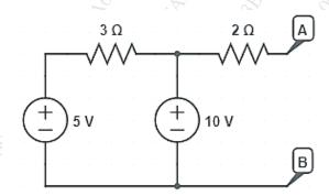
B) State and prove maximum power transfer theorem. Find the value of resistor (RL) that will transfer maximum power in the circuit given.
